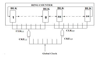
Fig.7. Tree structure clock tree drivers with gating in Octree system.
