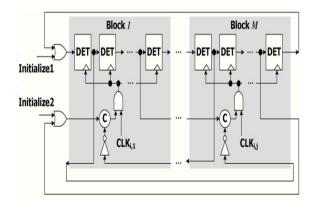
Fig.4. Ring counters with clock gated by C-elements
