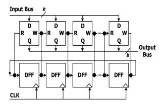
Fig. 2. Pointer-based delay buffer
