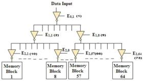
Fig.8. gated driver tree of input driving circuitry (Octree system)
