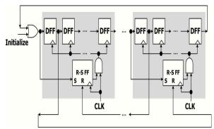
Fig. 3. Ring counter with clock gated by R–S flip flop
