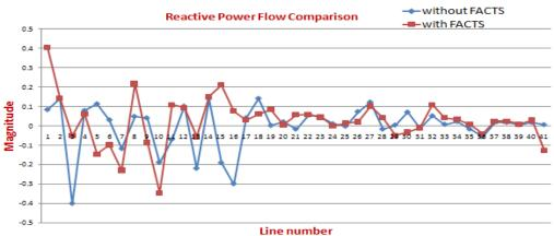
**Line number** Figure.10. 30% Over Loading Condition.
