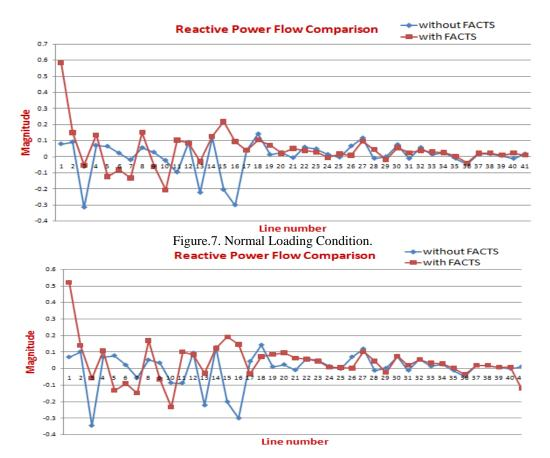
Figure.8. 10% Over Loading Condition.
