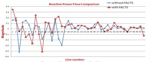
Figure.11. 40% Over Loading Condition.
