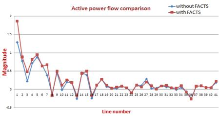
Figure.5. 40% Over Loading Condition.
