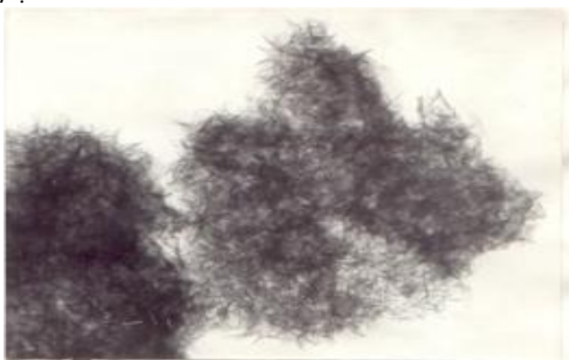
Figure.8 Transmission electron micrograph of unreduced catalyst showing fibrous state
