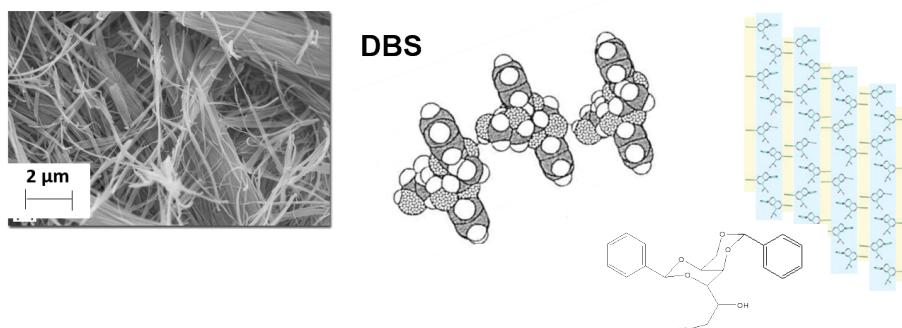
**Figure 3.** Schematic representation and scanning electron microscopy (SEM) micrographs of DBS (intra- and intermolecular hydrogen bonds,  $\pi\text{-}\pi$  stacking organization in organic medium).
