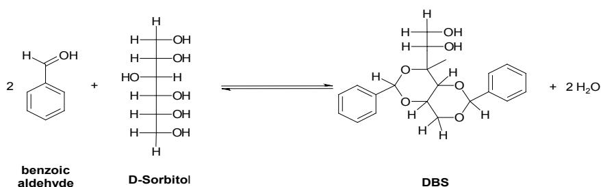
**Figure 4.** Synthesis of DBS molecules.
