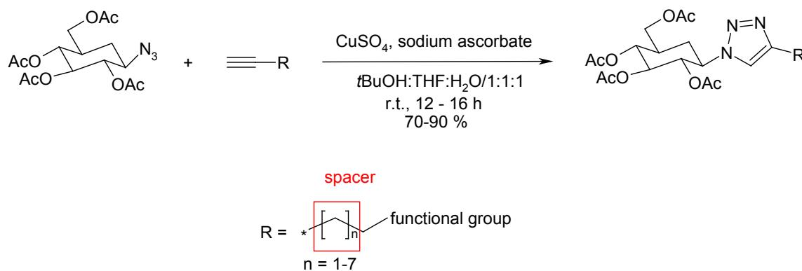
**Figure 7.** Synthesis of glucosyl triazole by the Copper-catalyzed azide-alkyne reaction [40].
