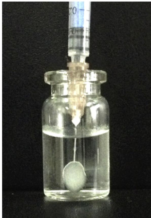
**Figure 12.** Instantaneous gelation of an organogelator injected in a 37°C solution [44].
