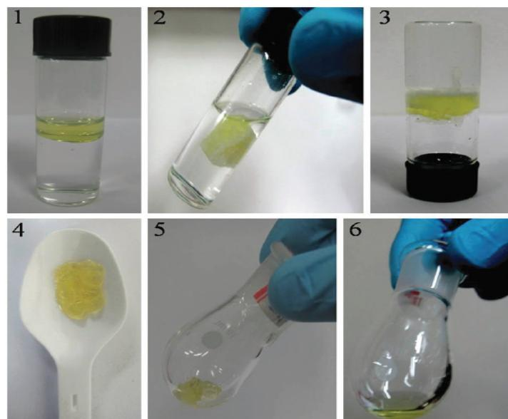
**Figure 13.** Selective gelation of the organic layer in a water diesel biphasic mixture at room temperature: (1) mixture of 2 ml water and 0.8 ml diesel, (2) gelation of the diesel layer instantaneously after addition of a solution of the gelator, (3) within 45 s the organogel is supporting its entire weight plus the weight of water in the inverted vial, (4) scooped organogel in spoon, (5) collected diesel gel in a round bottom flask, then (6) diesel recovered by distillation.
