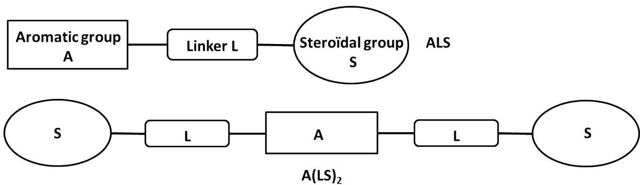
**Figure 2.** Graphical representation of Cholesterol-based organogelators; (a) ALS system containing aromatic group:linker: Steroidal group in rapport of 1:1:1, (b) A(LS)2 system containing aromatic group:linker:steroidal group in rapport of 1:2:2 [26].
