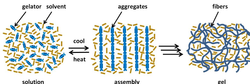
**Figure 1.** Schematic representation of self-assembly of organogelators in 3-Dimension fiber network [4].
