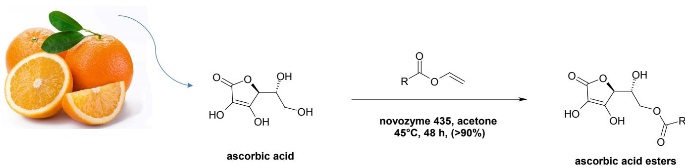
**Figure 11.** Representation of an enzymatic reaction basing on fruits biomass. Synthesis of ascorbic acid esters using a Novozyme<sup>[7]</sup>.
