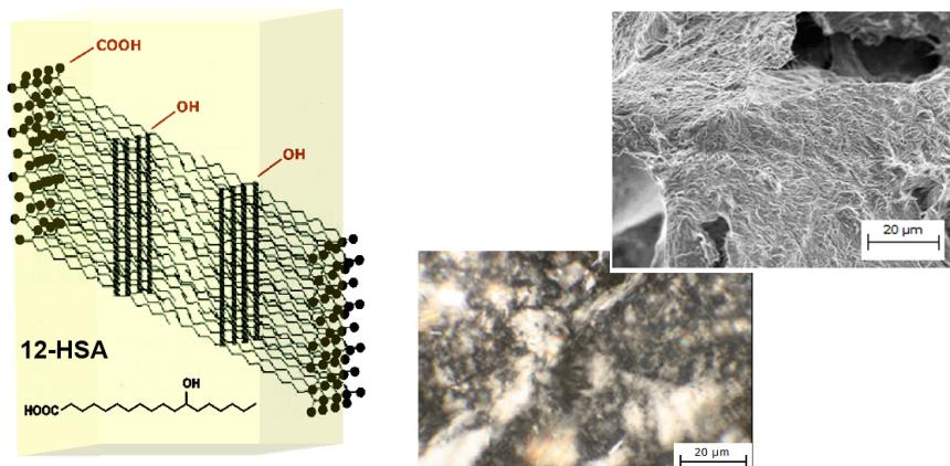
**Figure 5.** Schematic representation and scanning electron microscopy (SEM) micrographs of HSA (intermolecular hydrogen bonds, Van der Waals interactions).
