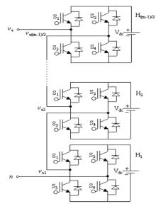
Fig. 1 Configuration of single-phase cascade multilevel inverter
