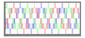
Fig. 8 Three phase output waveform of seven level cascaded inverter
