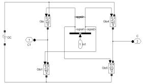
Fig. 6 Circuit diagram of sub system (H-Bridge)
