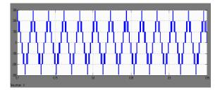
Fig. 7 Single phase output waveform of seven level cascaded inverter
