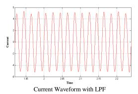
The total harmonic distortions of the system with filter are shown. The voltage THD of the system was reduced by 4.87 % as shown in Figure 8.3 and the current THD are reduced by 2.08% as shown Figure 8.4
