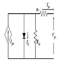
Fig.3 Single Diode Model of a PV Cell
