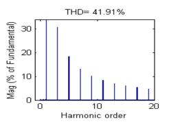
Figure 8.1. Voltage THD without Filter
