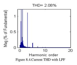
By using the PI controller and the LPF the THD of the system can be reduced as per IEEE-519 standards. The Table.2. gives the THD value of the system with and without filter added on the system.
