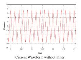
The total harmonic distortions of the system without filter are shown below. The voltage THD of system without filter is 41.91% as shown in Figure 8.1 and the current THD of the system is 8.91% are shown in Figure .8.2 In order to reduce the THD below 5% further the filters are used to bring it to the required standards.
