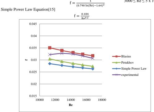
Figure 5: Comparison of present experimental friction factor with available correlations.
