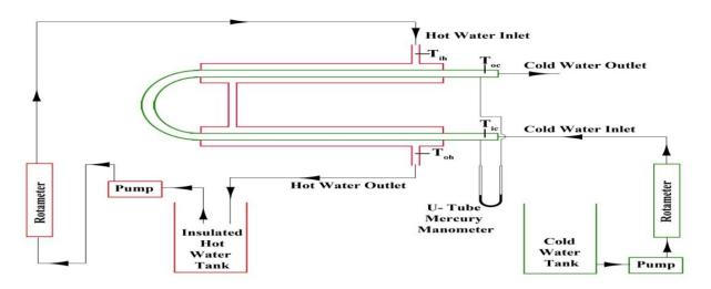
Figure2: Experimental Setup of Counter flow U-bend Double Pipe Heat Exchanger.
