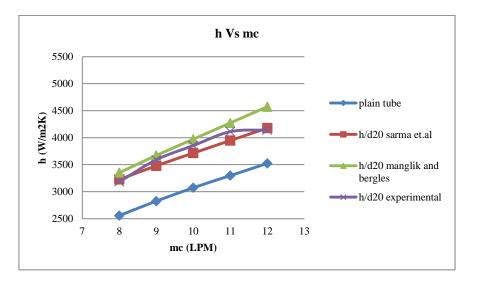
Figure 9: Comparison of experimental heat transfer coefficient with available correlations-twisted tape insert H/D 20.
