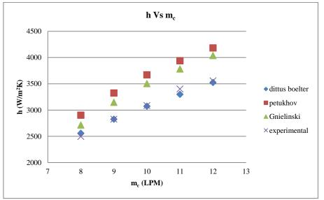
Figure 4: Comparison of present experimental Heat Transfer data with available correlations.
