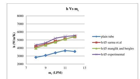
Figure 6: Comparison of experimental heat transfer coefficient with available correlations-twisted tape insert H/D5.
