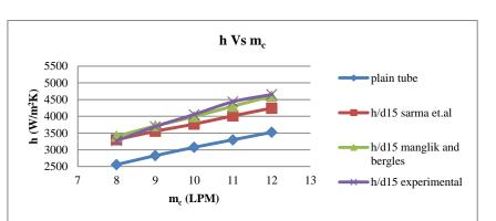
Figure 8: Comparison of experimental heat transfer coefficient with available correlations-twisted tape insert H/D 15.
