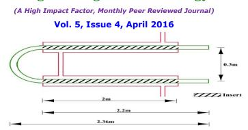
Figure1: Dimensions of U-Bend Double Pipe Heat Exchanger.
