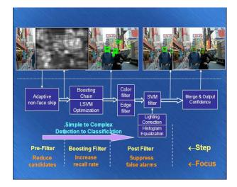
Figure 2. Face Detection System
