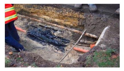
Figure 1: Example of underground cable fault.
