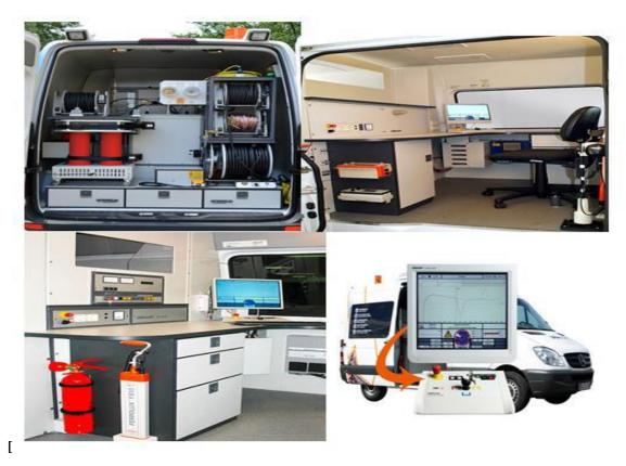
Figure 2: Centric system van for underground system cables faults.
