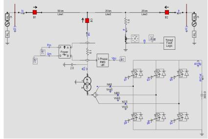
Fig. 3A transmission line with STATCOM at the mid-point modelled by PSCAD
