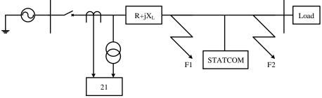
Fig. 1 Distance relay in a transmission system with a STATCOM at the midpoint
