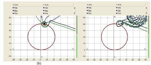
Fig. 10 Apparent impedance seen by distance relay during Three-phase fault (a) without STATCOM (b) with STATCOM
