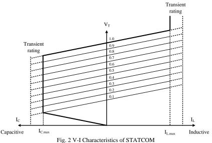
Fig. 2 V-I Characteristics of STATCOM
