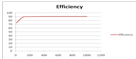
Fig 14. Input power Vs Efficiency of 81 level trinary proposed MLI
