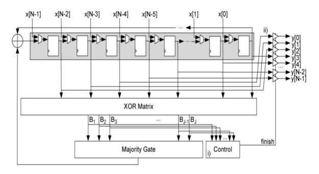
Fig. 3 Schematic Of The Proposed MLDD With Control Logic
