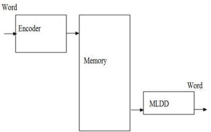
Fig. 2 Memory system schematic with MLDD
