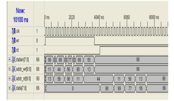
Fig.9 Simulation result of RAM
