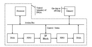
Fig.1 FPGA Coprocessor Architecture with DMA Controller in FPGA (Type F)
