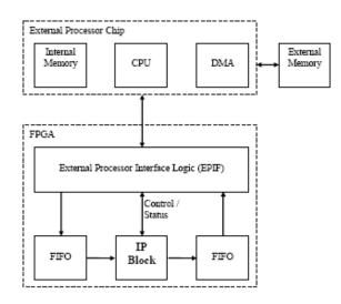
Fig. 2 FPGA Coprocessor Architecture with Off-FPGA DMA Controller (Type E)
