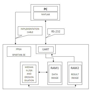
Fig.11 Block diagram of design implemented on FPGA
