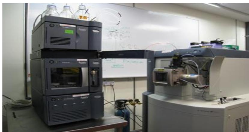
This UPLC technique takes full advantage of chromatographic principles to run the separation using columns which are packed with smaller particles and higher flow rate<sup>[29]</sup>. UPLC principal is based on the “Van Deemter equation” and it explains the relationship between flow rate and HEPT (height equivalent to theoretical plates) or efficiency of column<sup>[30]</sup>.
