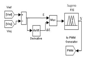
Figure. 4 Fuzzy controller in simulation
