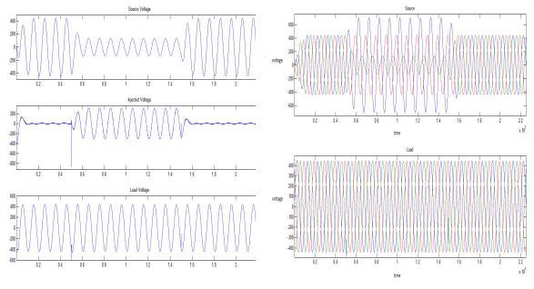
Figure. 7 Three phase source and load voltage
