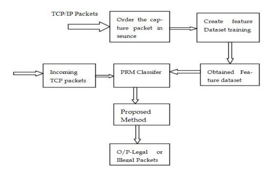
Fig .Block Diagram for covert channel detection
