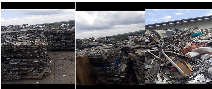
Figure 1. Figure shows prepared aluminium scraps for electrical conductor production at Bmet cable industry Ethiopia.
