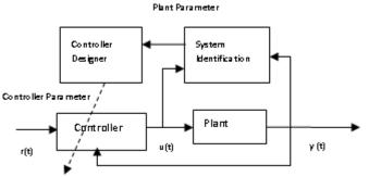
Fig.1 Indirect Adaptive Control using Takagi-Sugeno Fuzzy System
