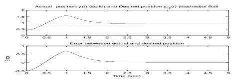
Fig.5 Variation of desired, actual angular position and their error magnitude for magnetic ball suspension system.
