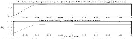
Fig.3 Variation of desired, actual angular position and their error magnitude for robotic manipulator.
