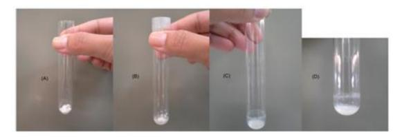
Figure 3: Tube containing (A) darunavir: $\beta$ -cyclodextrin (B) in phosphate buffer solution 0.05 *M* with 0.5 % Tween pH 3.0, (C) after 72 hours on shaker at 60 rpm and 37 °C ± 0.5 °C. (D) Detail of the presence of precipitate, ensuring saturation of the solution.
