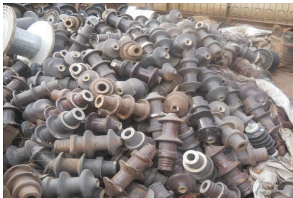
Fig. 2: Ceramic insulator bush waste dump at manufacturing industry
