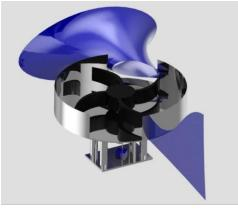
Fig. 5 CAD model of wind amplifier.
