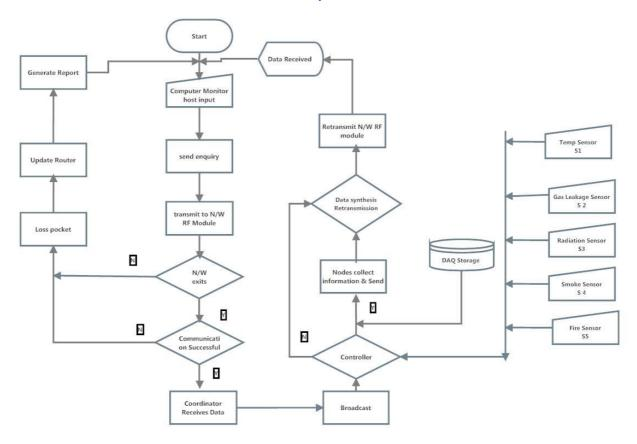
Fig 5: Software functional flow diagram
