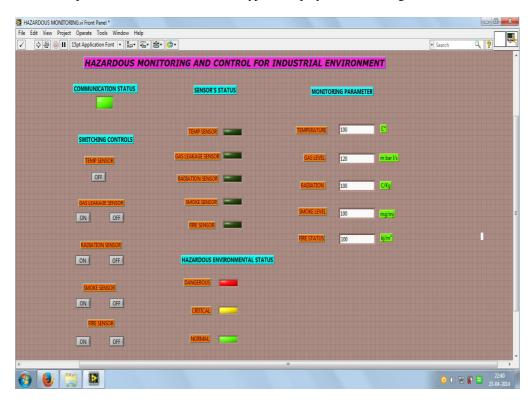
Figure 7: Experimental setup simulation using LabVIEW
