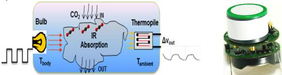
Figure 3: NDIR Gas Sensor Principle
