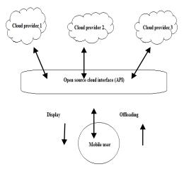
Fig 1.Architecture of Proposed Open Source Cloud API with Offloading
