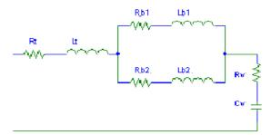
Fig2:Equivalent Electrical model of the respiratory system
