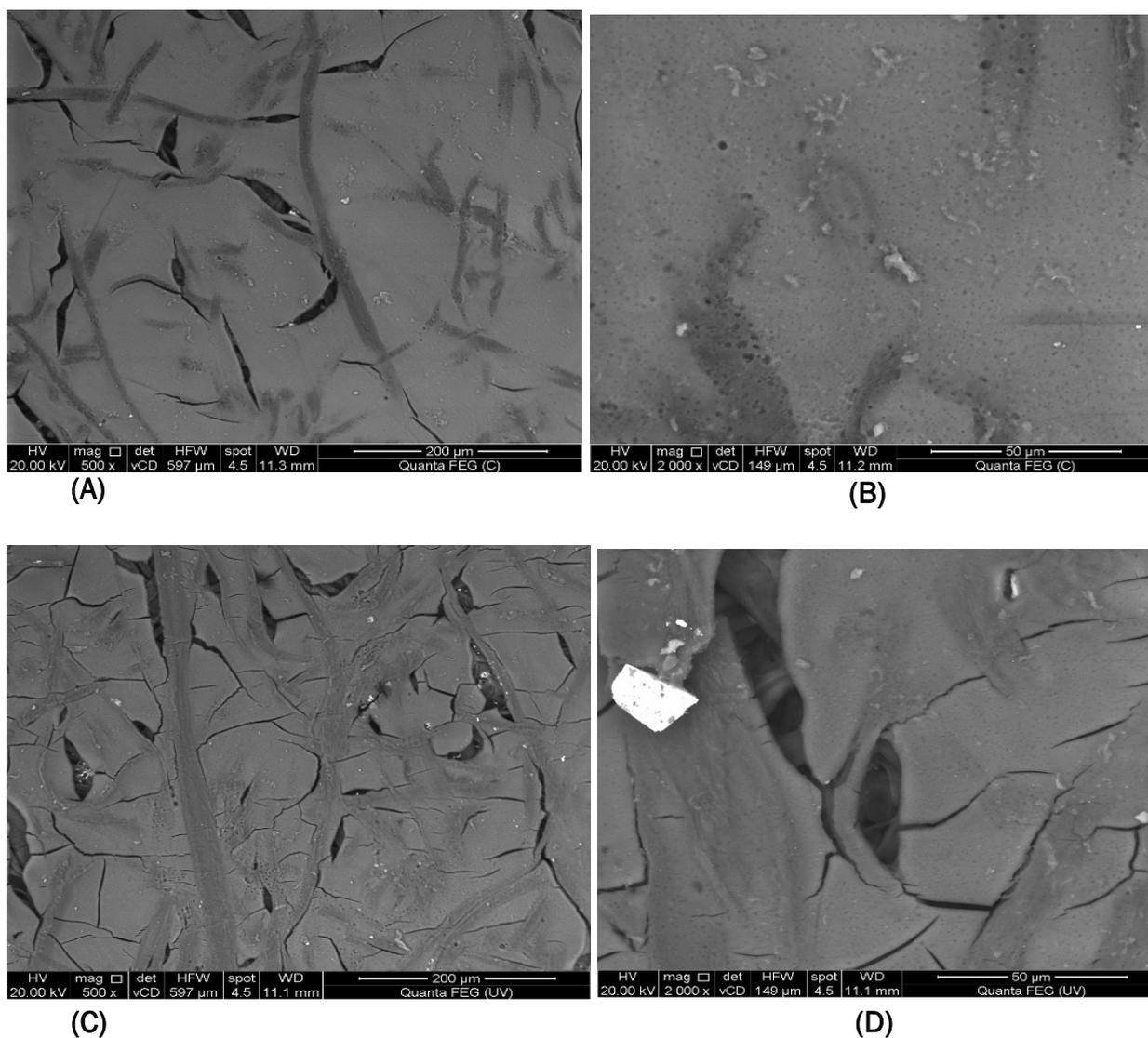
**Figure 1.** SEM photomicrographs of the silver albumen photographs sample: A: SEM photomicrographs (500X) and B: SEM photomicrographs (2000X) of samples before exposing to UV (Sb) we note serenity emulsion Albumen where impurities appear in Albumen clear; C: SEM photomicrographs (500X) and D: SEM photomicrographs (2000X) of samples after exposing to UV (Eb).
