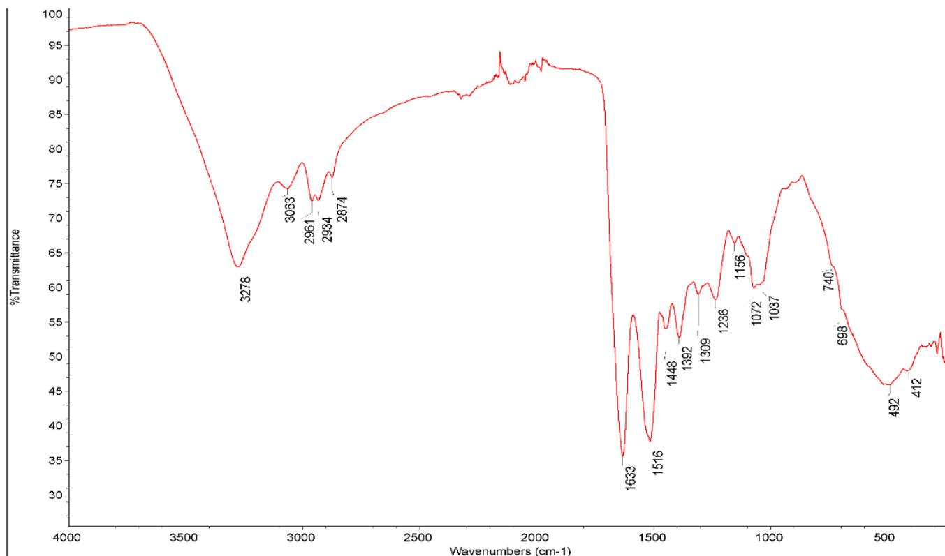
**Figure 3.** The IR spectrum of albumen on photographic paper is measured by ATR technique.
