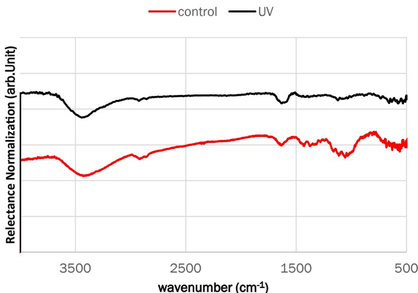
**Figure 4.** The IR spectra of albumen before and after exposure to UV beam in UVA band.
