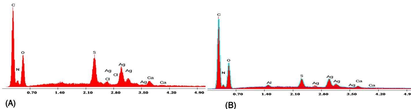
**Figure 2.** Analysis pattern of unit elemental analysis (EDX): A- shows the elements in the sample taken from the emulsion Albumen photo before the exposure to UV; B- shows the elements in the sample after.
