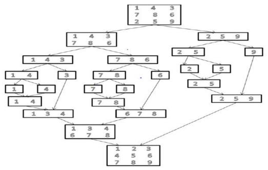
Figure 2. Dividing 3X3 matrix into sub matrices and Combining sorted sub matrices.
