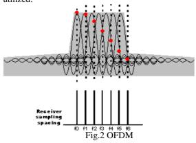
OFDM requires very accurate frequency synchronization between the receiver and the transmitter; otherwise it produces crosstalk between the subcarrier signals.
