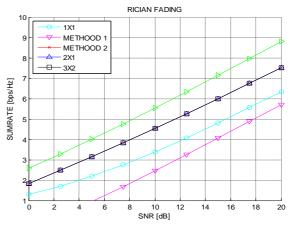
Fig.4.Sumrate for Various Methods Of Beamforming
