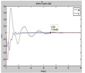
Fig. 5 Comparison graph of change in frequency of hydro-thermal power plant for PID to PI controller.
