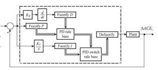
Fig. 2 The proposed multi stage fuzzy PID controller.
