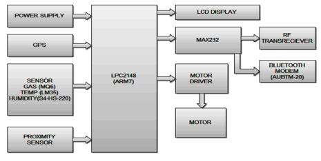
Fig.1. Block Diagram
