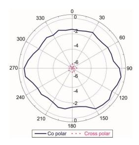
Fig. 3 Radiation pattern of SURMSA measured at 8.87 GHz
