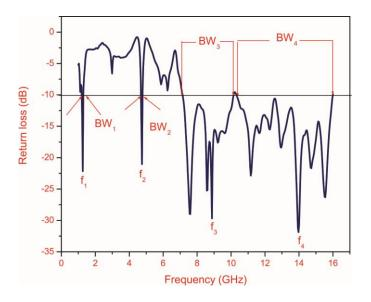
Fig. 2 Variation of return loss versus frequency of SURMSA
