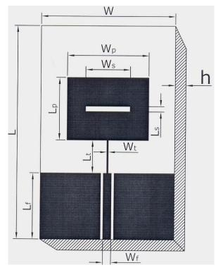
Fig. 1 Top view geometry of SURMSA
