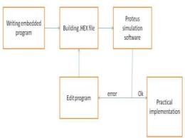
Fig.4 Block diagram of simulation steps
