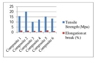
Fig.2 Comparision of Tensile properties of different composite laminates.
