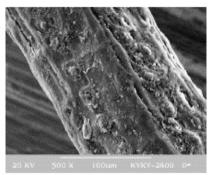
Fig. 4 Surface of untreated Coir fiber [1]
