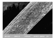
Fig. 5 Surface of coir fiber treated with NaOH solution.[1]
