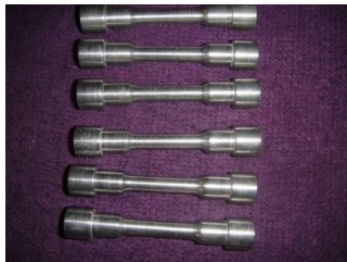
Fig.3.8: Tension test specimens
