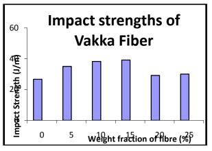
Fig. 8 Impact Strength of Vakka fiber / PP Composites at different weight fraction of fiber
