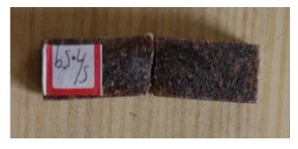
Fig. 3 Specimen after Impact Test The Impact strength is given by
