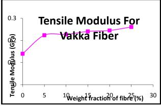
Fig. 5 Tensile Modulus of Vakka Fiber / PP Composites at different weight fraction of fiber
