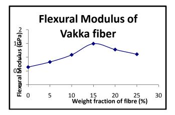
Fig. 7 Flexural Modulus of Vakka Fiber / PP Composites at different weight fraction of fiber
