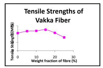
Fig. 4 Tensile Strength of Vakka Fiber / PP Composites at different weight fraction of fiber
