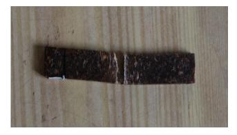
Fig. 2 A sample Specimen after Flexural Test
