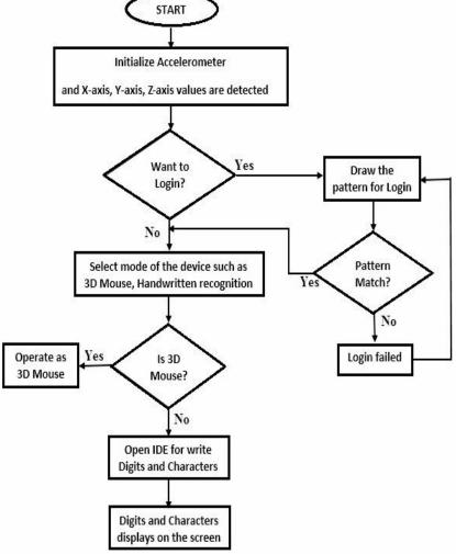
Fig. 4 Flowchart of MEMS accelerometer based system process
