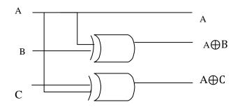
Figure.4 Combinational Circuit of Double Feynman gate
