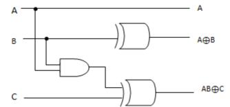
Figure.10 Combinational Circuit of Peres gate
