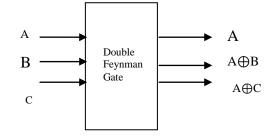
Figure .3 Block diagram of Double Feynman Gate www.ijircce.com
