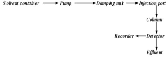
Figure 1: The various components of a HPLC system are herewith described
