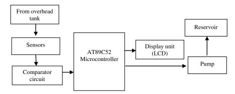
Fig.1. Block Diagram of the operations of the system
