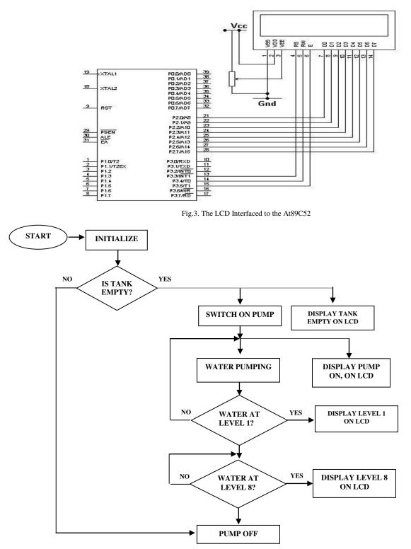
Fig.4. Flow Chart of the Automatic Water Level Monitor with Feedback
