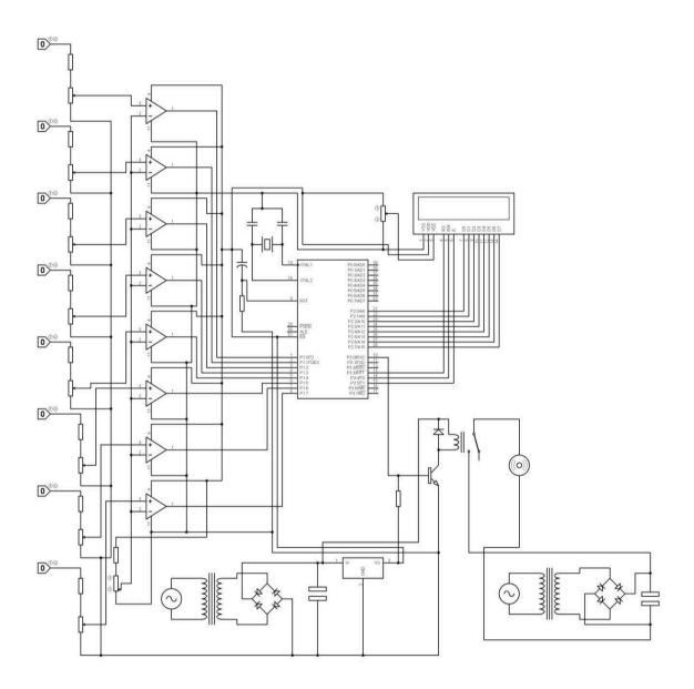
Fig.5. Schematic Diagram of the Automatic Water Level Monitor with Feedback
