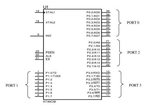
Fig 2. I/O Port Pin and microcontroller connection diagram
