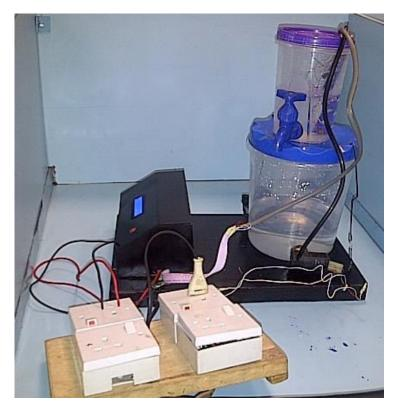
Fig.7. Hardware Prototype of the automatic water level controller
