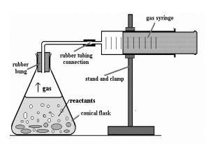
Fig. 2 Experimental setup to determine the rate of decomposition without the addition of catalyst
