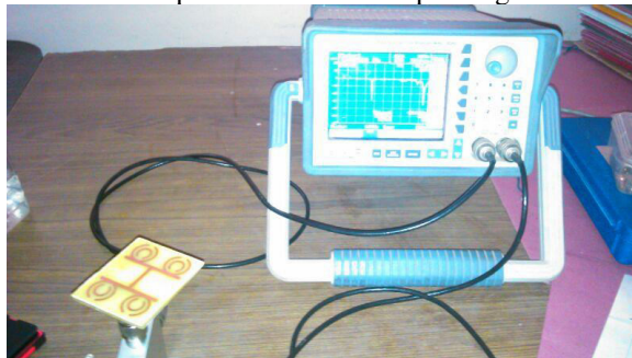
Figure 13: Measurement of reduced size antenna loaded with “H shaped interconnected split ring” Metamaterial antenna.
