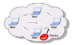
A distributed protocol, called UNMASK, for detection, diagnosis, and isolation of nodeslaunching control attacks, such as, wormhole, Sybil, rushing, spoofing, and replay attacks. UNMASK uses localmonitoring to detect control and data traffic, and local response to diagnose and isolate the Thesaurusnodes.
