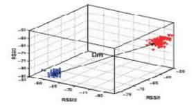
Fig.1. Illustration of RSS readings from two physical locations.
