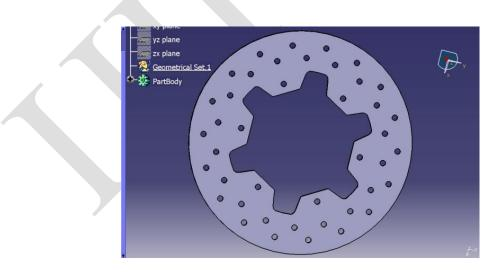
Fig.2.1 Disc Brake Model in CATIA
