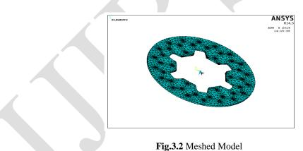
The above figure is the meshed model in the ANSYS analysis for the structural analysis. In this meshed model triangular type meshing is used for the solid disc brake in the analysis procedure. In this regular type meshing is done in the analysis process.
