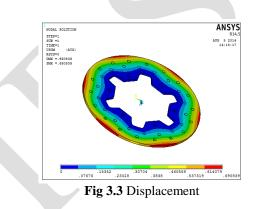
The above shown figure is the Displacement diagram of the Aluminum obtained in the stress analysis in the ANSYS process. In the Aluminum stress analysis, Displacement minimum load is 0.00000 and the maximum load is 0.690839. It has the maximum load when compared to the remaining materials Grey Cast Iron, HSS M42 and HSS M2.
