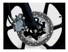
Fig.1 Assembly of Disc Brake
