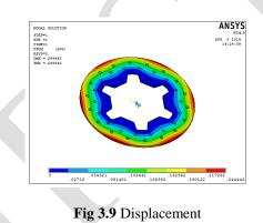
The above shown figure is the Displacement diagram of the HSS M42 obtained in the stress analysis in the ANSYS process. In the HSS M42 stress analysis, Displacement minimum load is 0.00000 and the maximum load is 0.244443. It has the second minimum load when compared to the remaining materials Aluminum, Grey Cast Iron and HSS M2.
