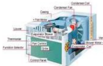
Figure 2. Air conditioning system.
