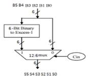
Fig.3, 6-b BEC with 12:6 mux.
