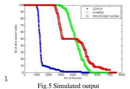
In Fig. 5, a detailed view of the behaviour of HEED and H-HEED protocol is illustrated; it shows the number of alive nodes per round. The number of nodes death in HEED is more than H-HEED over the same number of rounds. The number of normal nodes dies very fast and as a result the sensing field becomes sparse very fast. On the other hand, due to the higher energy than the normal nodes the advanced nodes and super nodes die slowlyBut in multi-level H-HEED,
