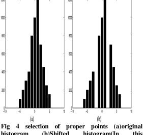
histogram (b)Shifted histogram(In this figure,length of messages is 1000 bits,LP=-2 and RP=2)
