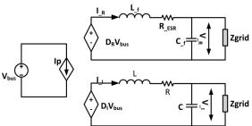
Fig. 5. Average circuit model in the *RI* stationary frame.
