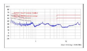
Fig. 15. Conducted emissions spectrum of the micro inverter with passive EMI filter..
