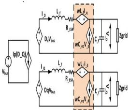
fig.6 Equivalent circuit model in the DQ rotating frame
