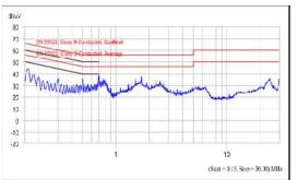
Fig. 17. Conducted emissions spectrum of the microinverter with DAEF installed.
