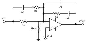
Fig 11. Schematic diagram of the type III compensator.
