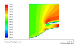
Figure 6 contours of velocity magnitude
