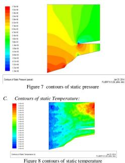
The above scram jet combustor model has been analysed by using FLUENT which has produced the velocity and pressure variations by generating the contours of velocity and pressure and also the temperature. By these variations in velocity and pressure, the turbulence mixing can be analysed with shock wave interacted in the combustor before injecting the fuel.
