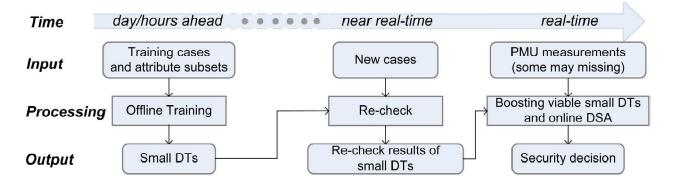
Three-stage ensemble DT-based approach to online DSA with missing PMU measurements.:
