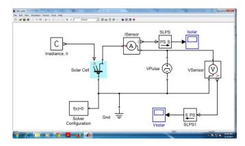
Figure 3.MATLAB & Simulink model for analyzing solar cell voltage and current
